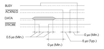
Transition time (both the rise and the fall) of every signal must be less than 0.2  $\mu s. \,$
